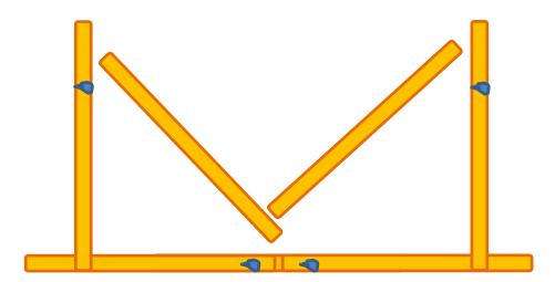
Using two more craft sticks, glue braces on either side of the frame, as shown above.
